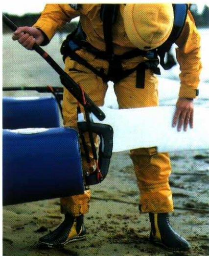
Dart's new rudder system uses a simple rubber band as a locking mechanism...
